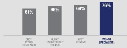
Test evaluates the cleaning ability of a fluid using a mechanical device. Score shows percent of soil removed.
