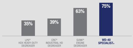
Test evaluates the cleaning ability of a fluid using a mechanical device. Score shows percent of soil removed.
