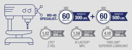
Test measures length of lubrication under pounds of force before breakdown.
