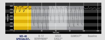
Results show average RPM after products are applied and recorded for standard deviation from the average. Closer to baseline and smaller standard deviation is better as these imply minimal stalling effects.
